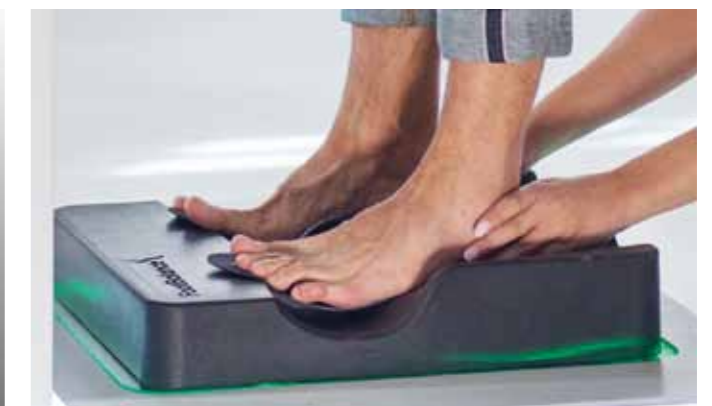
4. The heated insoles are moulded to each foot individually, whilst keeping the customer's feet in the correct alignment.
