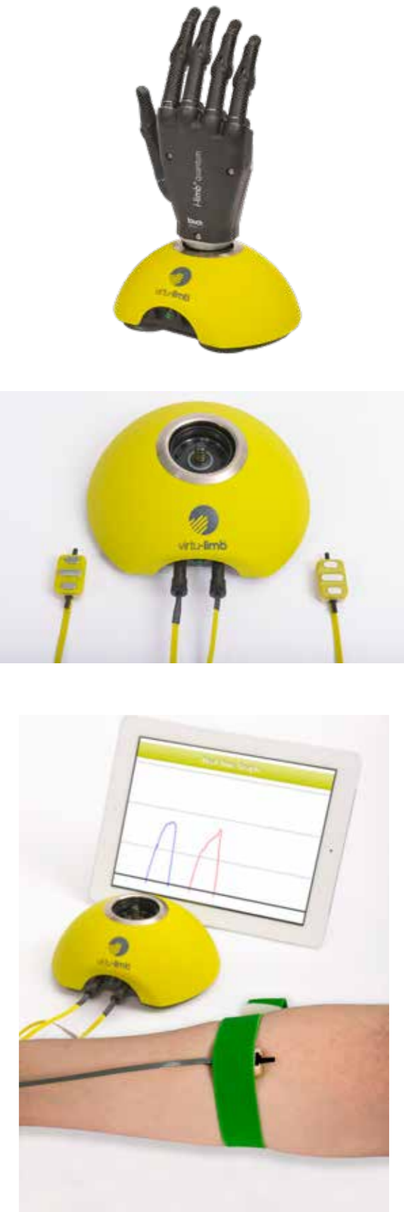
virtu-limb™ to measure myoelectric signals
